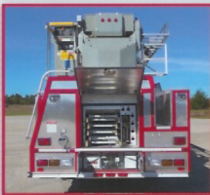
ENCLOSED GROUND LADDER STORAGE
